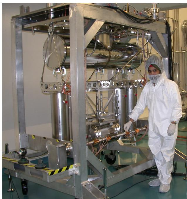
Figure 5 The cryomodule components in the assembly stand. The WPM system is in the foreground.
